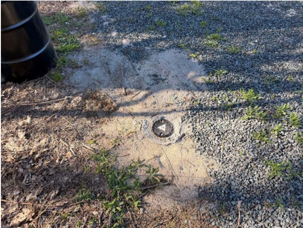
Photo 9 - Recent test boring
